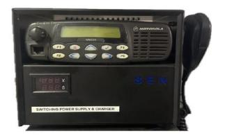
This device is designed and manufactured to convert a mobile Radio to base station Radio. long-term and reliable work is provided for this device by taking into account the basic protections for it. for installing the Radio, it is necessary to open the door of the device and fixing the Hytera or Motorola Radio to the bracket using provided screws.
